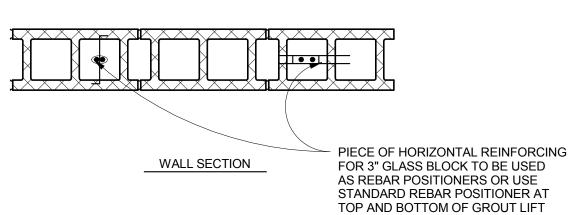
TYP REINFORCEMENT MASONRY VERTICAL LAP SPLICING DETAIL SCALE: N.T.S.
