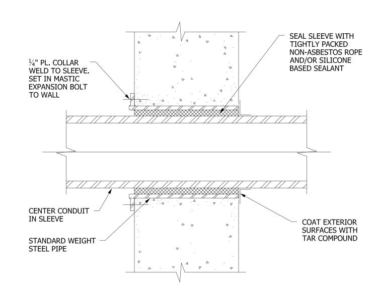
CONDUIT THROUGH EXISTING **EXTERIOR WALL** NOT TO SCALE
