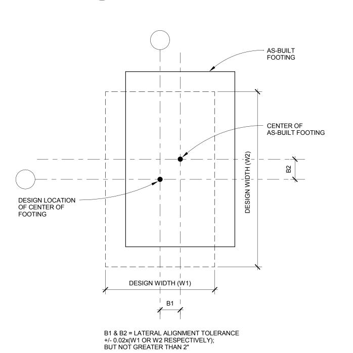
TYP SPREAD FOOTING PLAN TOLERANCE
