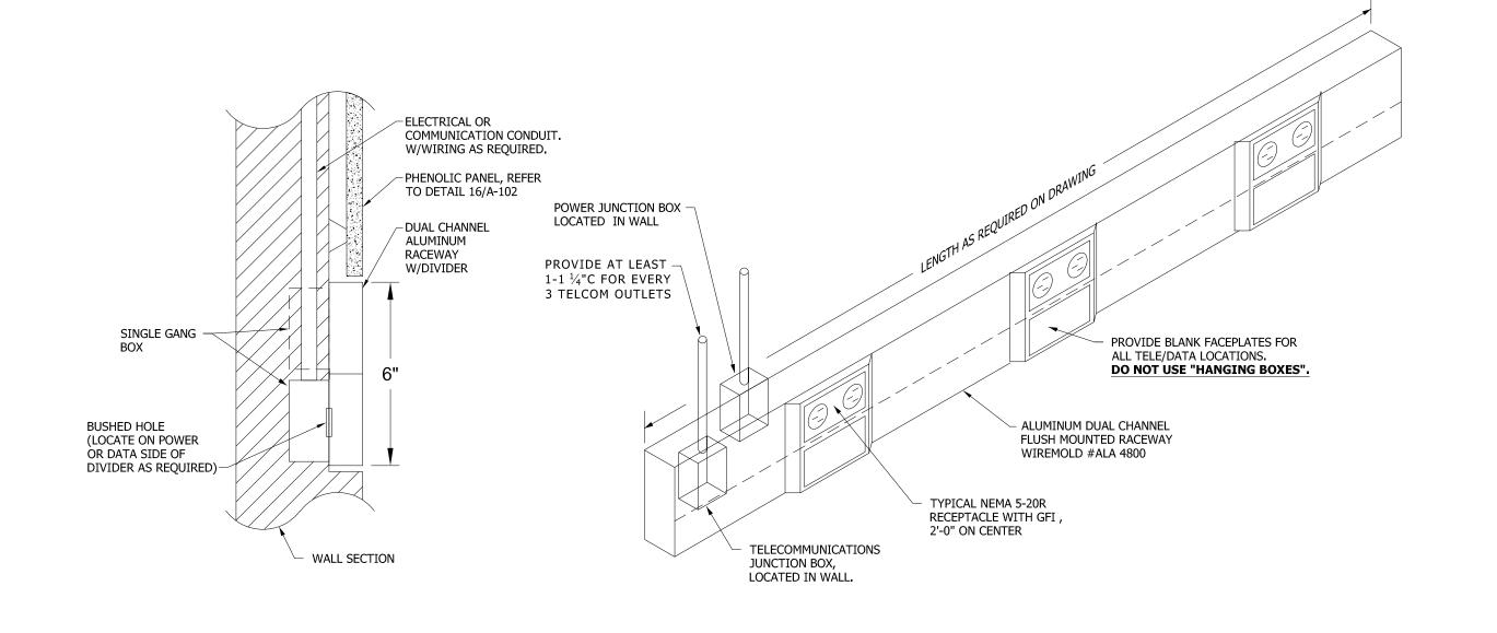
INSTALLATION DETAIL - FOR NEW WALL DUAL CHANNEL METAL FLUSH RACEWAY NOT TO SCALE
