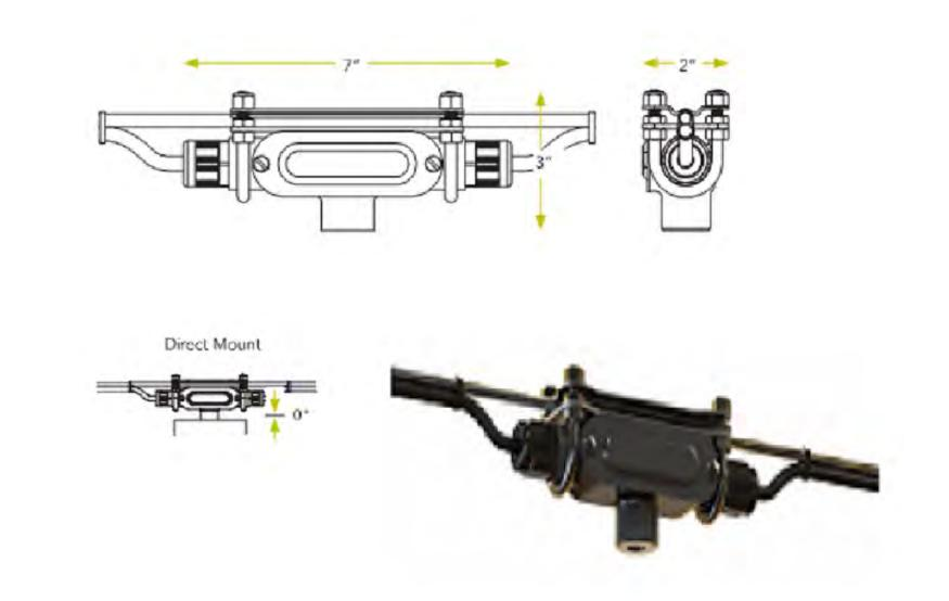
CATENARY MOUNTING DETAIL FOR TYPE "L1" LIGHTING FIXTURE
