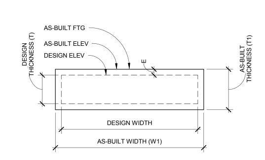
E= ELEVATION TOLERANCE (TOP OF FTG):
