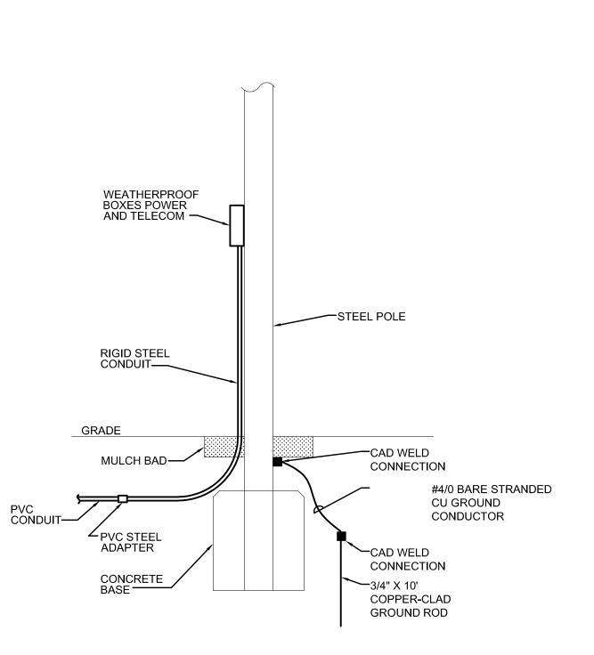
TYPICAL DETAIL FOR DEVICES MOUNTED ON STEEL POLE
