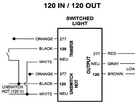
THE EMERGENCY INVERTER UNIT UPON FAILURE OF NORMAL POWER PROVIDES EMERGENCY POWER TO THE CONNECTED LIGHTING LOAD FOR A MINIMUM OF 90 MINUTES REGARDLESS OF LOCAL SWITCH POSITION. IT SHALL ALLOW CONNECTED LIGHTING TO BE ON, OFF SWITCHED OR DIMMED WITHOUT AFFECTING THE EMERGENCY OPERATION. INVERTER TO BE UL924 LISTED FOR REMOTE INSTALLATION UP TO 1000FT FROM THE EMERGENCY FIXTURE.
