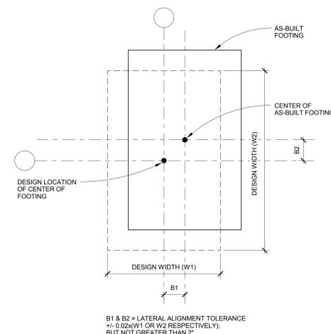
1 TYP SPREAD FOOTING PLAN TOLERANCE
