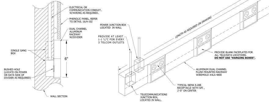
INSTALLATION DETAIL - FOR NEW WALL
