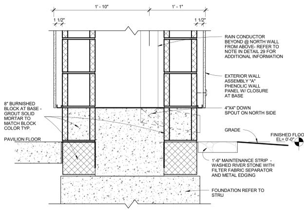
25 MASONRY CAVITY WALL ASSEMBLY
