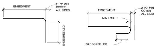
10 TYP CONCRETE REINFORCING BAR STANDARD TENSION HOOK (3000 PSI)
