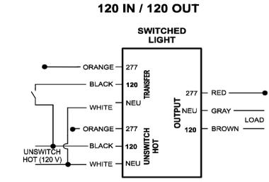
EMERGENCY INVERTER WIRING DIAGRAM
